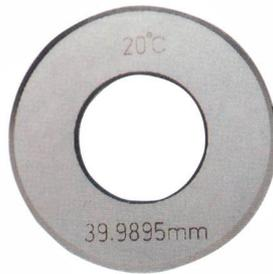
Setting Rings can be used to set Dial Bore Gauges, Tests, the inside of Micrometers, and other bore measuring instruments accurately and quickly. All setting rings are engraved to 0.0001mm with the actual calibrated size. When selecting a measuring ring, please choose one that is closest in size to the dimension to be measured and that falls within the measuring range of your instrument.
