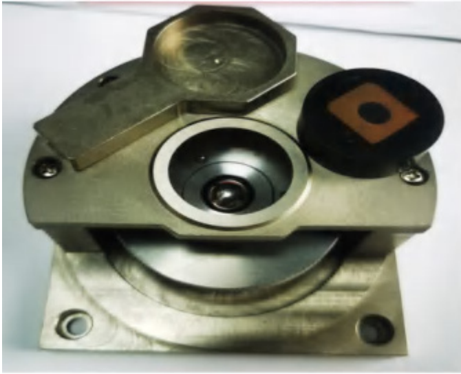
Single Inlay Sample Clamping
