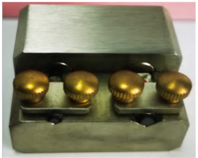
Pencil Clamping (For Pencil Hardness Test)
