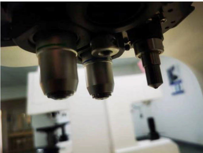
One Indenter with Two Objective System
