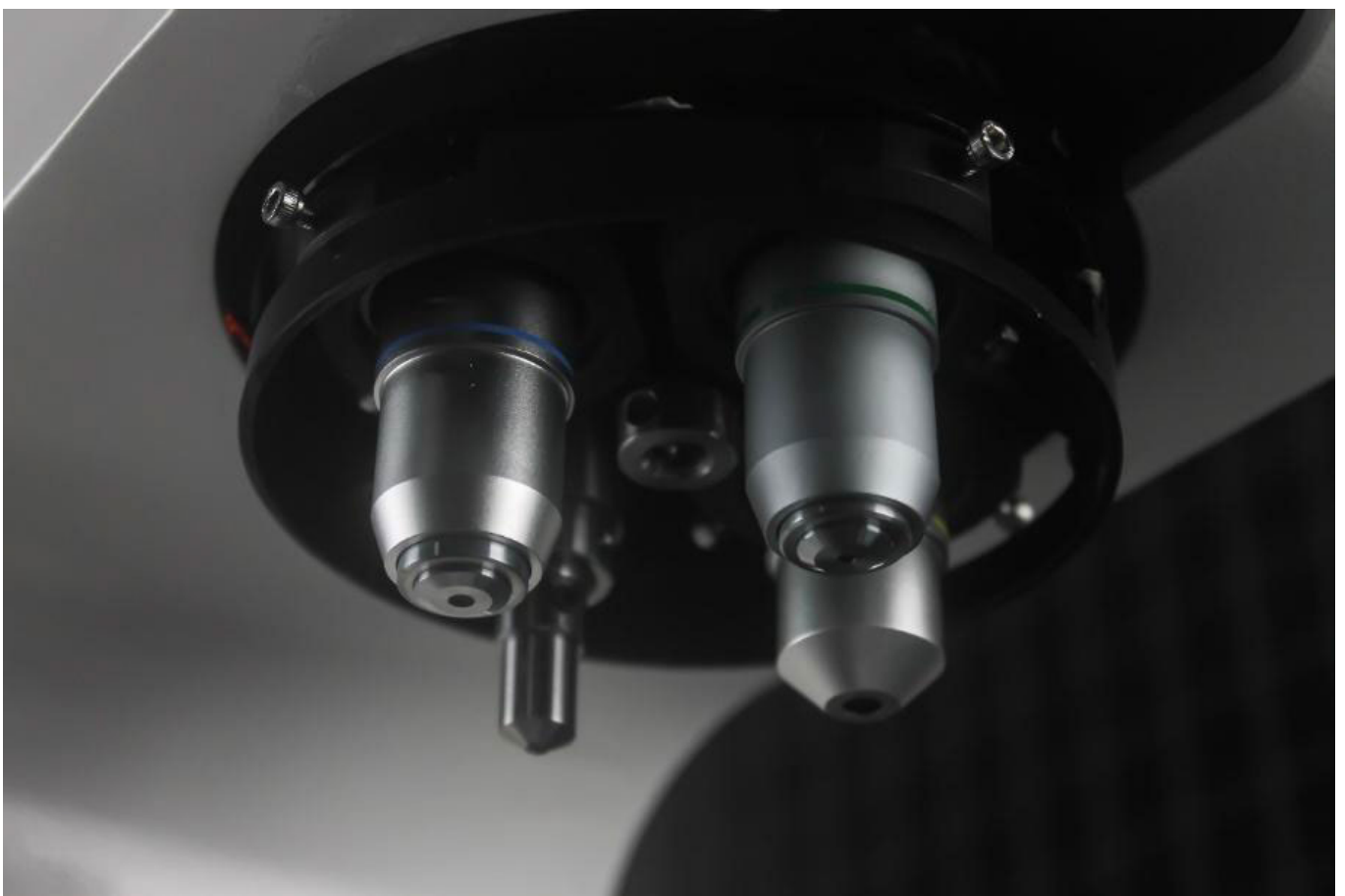
One Indentor with Three Objective Lens Realized
