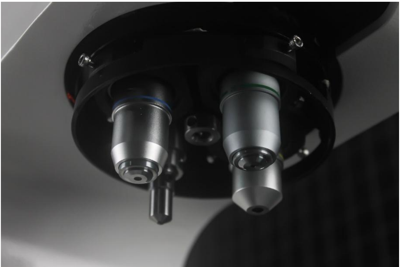
One Indentor with Three Objective Lens Realized
